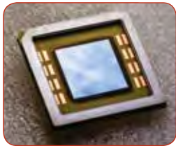
Uniform flip-chip silicon thinning
