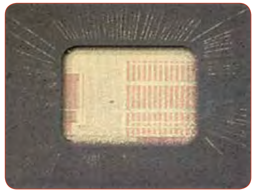
Pre-chemical decapsulation - Cu bond wire
