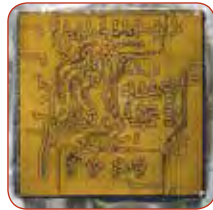
Uniform FR4 substrate delayering
