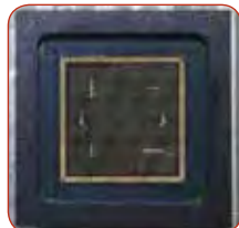
Uniform copper (Cu) pillar deprocessing - molded package, stacked die
