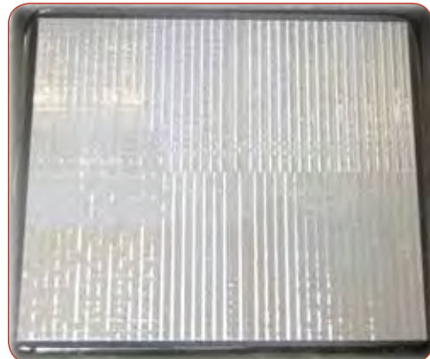
Deprocessing the device by following its profile ensures uniform material removal.
